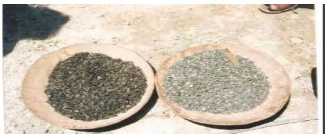
Fig 20 Mixture of platic and fine aggregate
